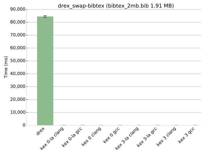
Figure 5.25: Execution time of the program drex_swap-bibtex on 2 MB of input data.
